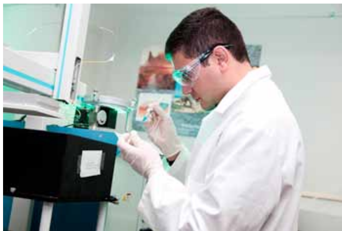
UA graduate student Miguel Etayo-Cadavid uses a syringe to inject acid into a vial containing samples for isotopic analysis.
