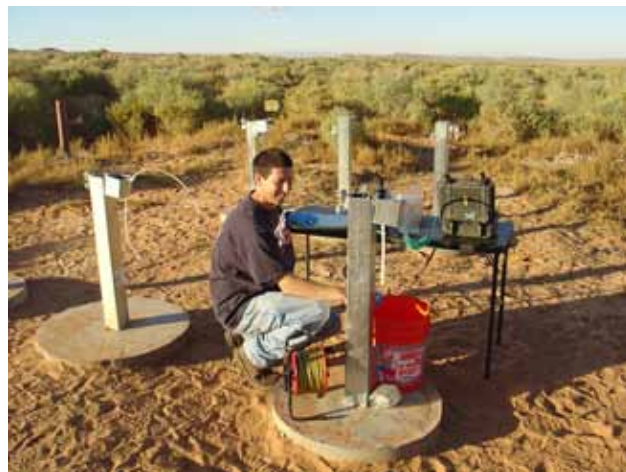
Photos above and below: Field Scale Remediation Project at DOE Monument Valley Uranium Mill Tailing Site: Monitoring the injection of ethanol and tracer and sampling nitrate concentrations in the aquifer.
